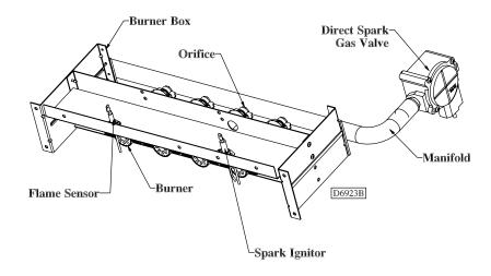
Figure 2 Heat Exchanger Details
